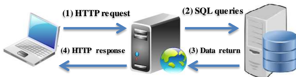
Figure 2.2: Web application with server and a back-end database.
